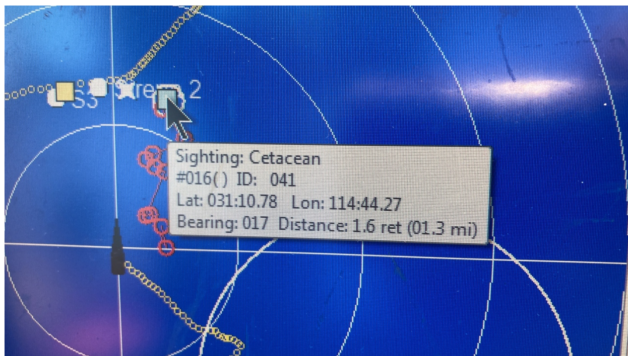
Figure 6. Screenshot of sighting 16. The black ship in the center depicts the position of the Seahorse with its path shown by yellow circles. The path of the mother/calf pair of vaquitas is in red open circles with the last position shown where the cursor is pointing and in the text box. The Sirena is located at the yellow box. Each white circle is a nautical mile (1.85 km).
